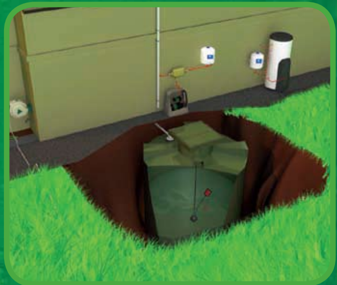
In ground tank, surface mounted pump with pump cover, wall mounted Rainsaver MKIII. Shown with optional energy saver pressure tank.
